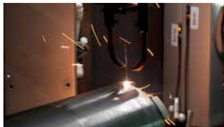
Laser welding of core drills.
