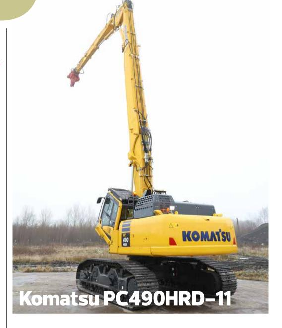
The new PC490HRD-11 is the latest in Komatsu's range of heavy duty demolition excavators. It brings what the company claims to be 'a best in class' working height to the 60t machine sector, and can be configured in six different working arrangements. It carries a 2t demolition tool up to a height of 32m, a 3.34t tool up to 28m and it can work with a 5t demolition tool up to 17.4m, enabling operators to work through the widest possible range of activities with optimal control and safety.
