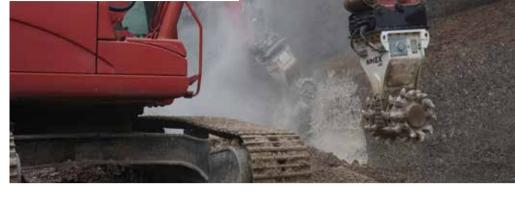
novative system with a central chain that leaves no areas unmilled, enabling the attachment's working capacity to be exploited to the maximum. Especially suited to nursery and forestry applications, such as cutting trunks and roots, these attachments prove highly effective for digging small trenches on rocky terrain or excavating small manholes or utility vaults for water, telephone or electrical lines.
