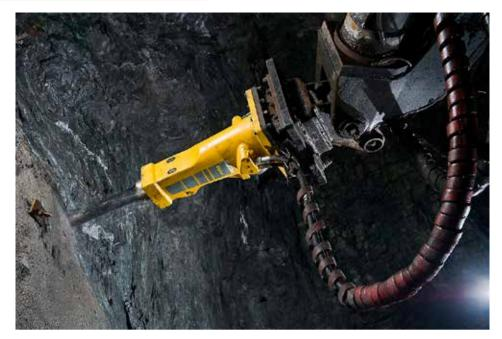
60 machine, all the way up to the 700kg BHB 705 for the recently introduced Brokk 500 and Brokk 520D. The attachments are lightweight and compact, yet feature power similar to larger, heavier breakers from other manufacturers. The hammer bodies are machined from a solid casting, eliminating side and through bolts, along with the side plates found on many other hammer designs. An integrated, side mounted accumulator holds a nitrogen gas charge for as long as a year.
