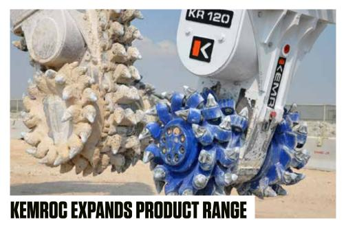
Kemroc, the manufacturer of excavator attachments, has announced a major expansion to its product range, including a complete range of twin head rotary drum cutters.
