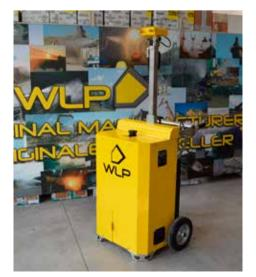
of dangerous bacteria with the aid of non-toxic additives, a self-contained NCA system consists of an electric generator set, a large volume tank with decontamination solution and a spraying cannon or nebulizer. Thanks to the on board electronics and a radio controlled unit, the system can be operated in remote mode, which drastically reduces the risk of the operator being infected. Complete autonomy and the ability to treat large areas are further benefits of the WLP solution.
