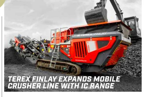
The IC range of compact impact crushers comprises of the IC-100, IC-100RS, IC-110 and IC-10RS models, all specifically designed for quarrying, construction and demolition debris, reinforced concrete and asphalt recycling applications.
