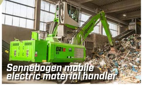
Configured as a mobile version, a Sennebogen 821 E is being used to feed one of Germany's most modern waste sorting facilities operated by Hufnagel Service. The family run waste management company opted for the material handler which is connected to the power supply via a permanently installed cable on the ceiling of the hall. Additionally, the diesel generator replaces the rear ballast, with the diesel power pack being able to be removed for maintenance work.
