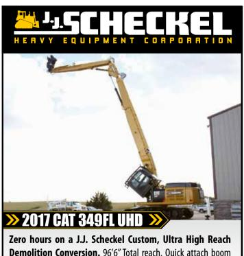
**Zero hours on a J.J. Scheckel Custom, Ultra High Reach Demolition Conversion.** 96'6" Total reach, Quick attach boom and lines, Hydraulic tilt cab, Extra counterweight, Highest quality package. Optional Cat MP324 multi processor tool and jaw sets at additional price if needed. The stock boom, stick, and bucket are also available if needed at additional price. **\$458,000**
